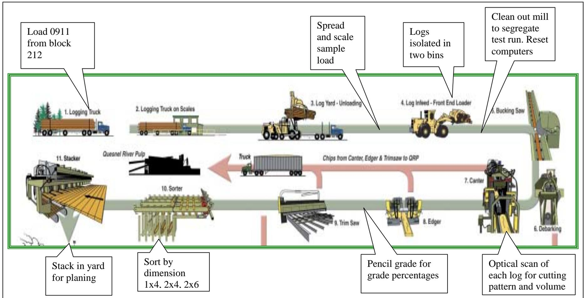
Figure 4: Schematic representation of West Fraser Timber Ltd. mill flow, showing critical points for conversion testing.
