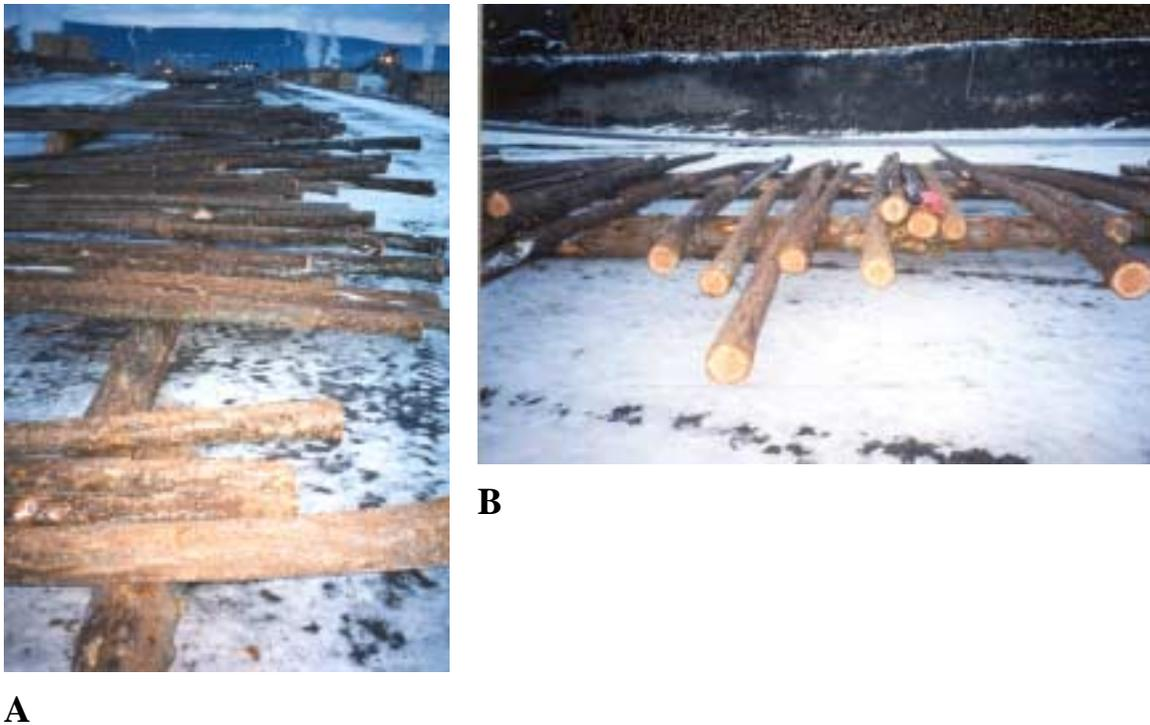
**Figure 3: Sample load 0911 spread for stick scaling before conversion test at West Fraser Timber Ltd. Williams Lake. Note short length and sweep (A) and small diameters (B) of the logs.**
